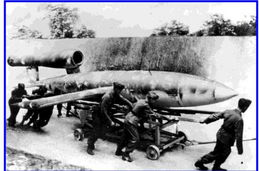
The engine ignited at around 50 times a second and produced a pulsing sound, and it became known as the Buzz Bomb. It could perhaps be considered as an early version, of today's cruise missile.
